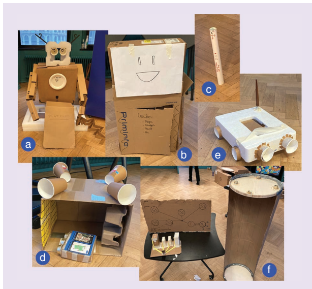
FIGURE 3. Cardboard prototypes for urban service robots. (a) Public assistant robot, (b) personal help desk assistant, (c) guiding tool at municipalities, (d) Public Transportation Guide & Hub, (e) underfloor maintenance surveillance robot, and (f) tools and concept for clean water management.
